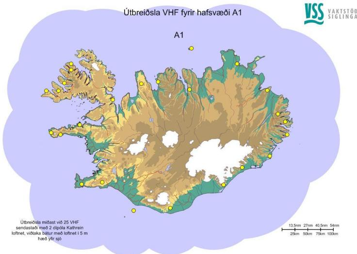
VHF coverage on Sea area A1 based on 25 VHF stations and recipient antenna at 5 m above sea level.
